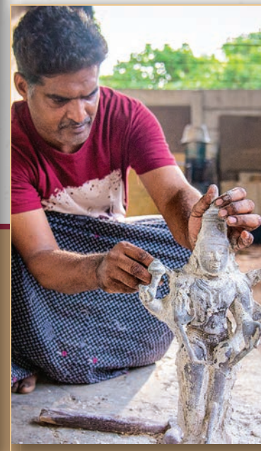
(counterclockwise from far left) pouring molten metal into the empty mold after the wax was melted out; artisan Suresh Subramanian scrapes remaining clay off the murti; final chiseling and polishing of a Ganesha murti
