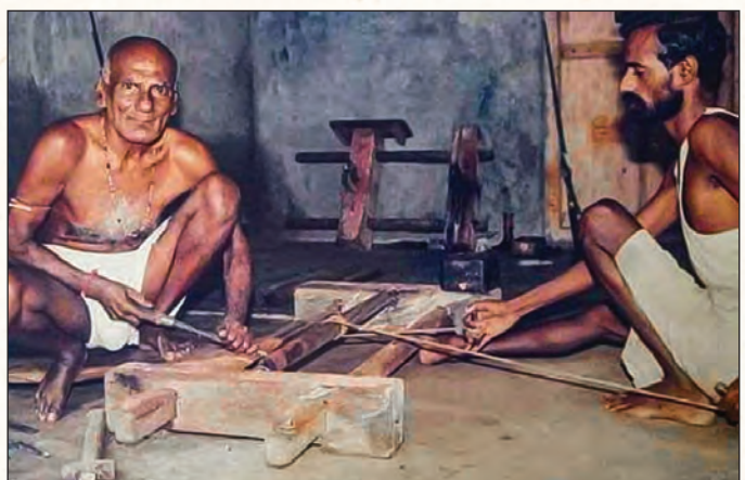
Sound craft: (left) a variety of nagaswaram styles; (above) N.G.N. Ranganatha Asari at his workshop in Narasingampettai. They are operating a rustic lathe; the master cutting with a chisel while his helper spinning the blank with a handled cord.
